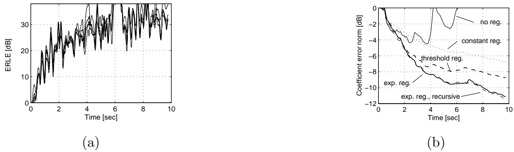
Fig. 11. (a) ERLE convergence for the multichannel cases P=2,3,4,5 and adjusted \alpha and (b) comparison of regularization methods, P=5 , \alpha=16 .
