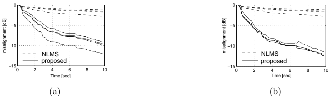
Fig. 10. Misalignment convergence for the multichannel cases P=2,3,4,5 . (a) Overlap \alpha = 4 , (b) overlap \alpha adjusted.
