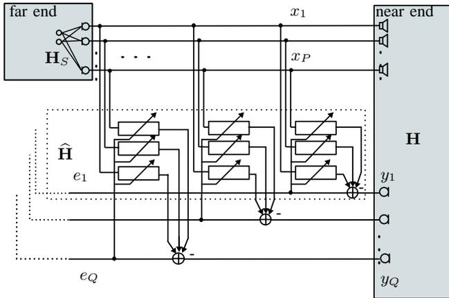
Fig. 1. Block diagram of multichannel acoustic echo cancellation as a prominent example for adaptive MIMO filtering.
