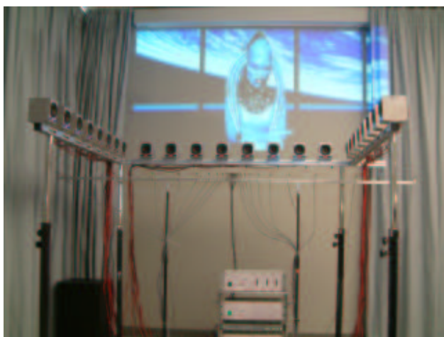
Fig. 3. 24-channel loudspeaker array and 26-channel microphone array in a multimodal full-duplex communication interface.
