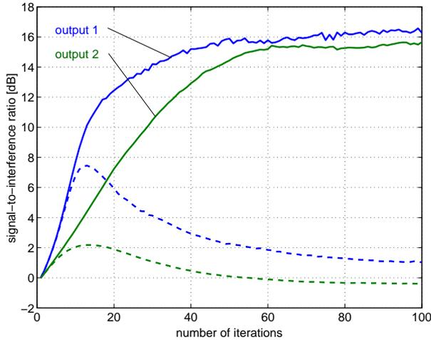
Figure 5: BSS performance of the wideband approach (solid) and the narrowband approach (dashed).
