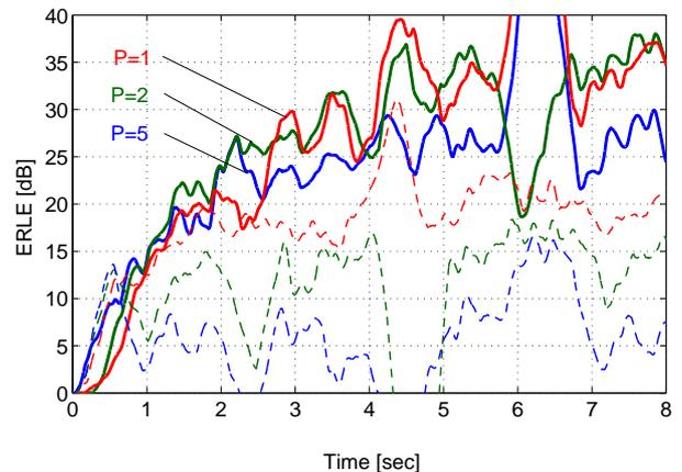
Figure 4: MC-AEC performance of the wideband approach (solid) and the narrowband approach (dashed).
