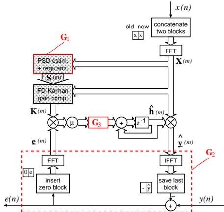
Figure 3: Generic SISO supervised FDAF as an example for the wideband approach.
