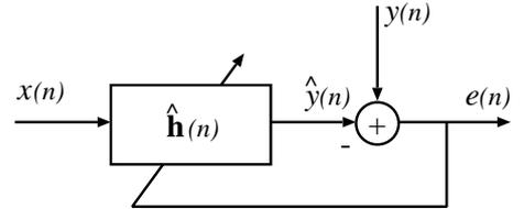
Figure 1: Single-channel supervised adaptive filter.
