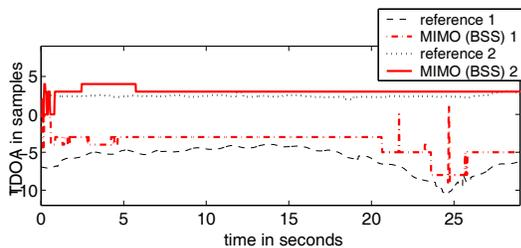
Fig. 4. Simultaneous TDOA estimation for two sources.
