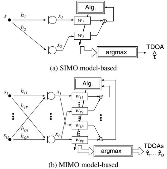
Fig. 1. TDOA estimation via (a) SIMO and (b) MIMO model-based blind adaptive filtering.
