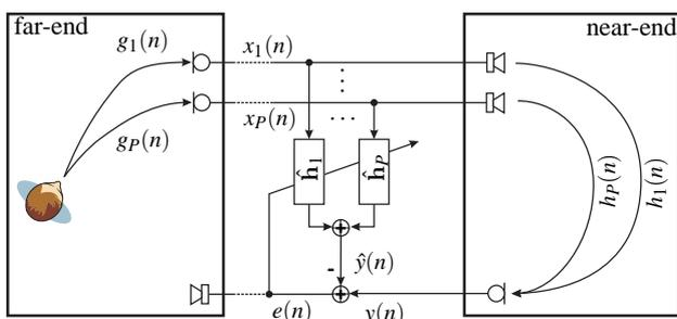
Figure 1: Block diagram of multichannel acoustic echo cancellation.
