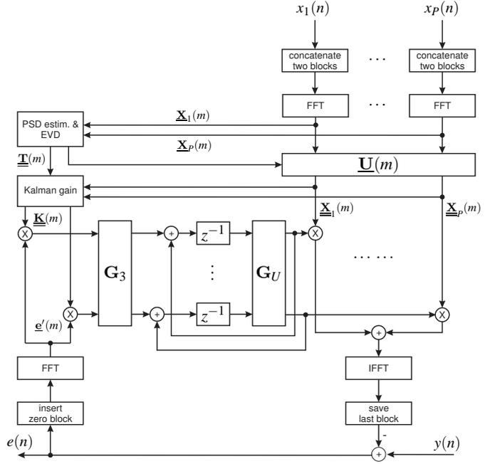
Figure 2: Block diagram of TDAF algorithm (adapted from [7]).
